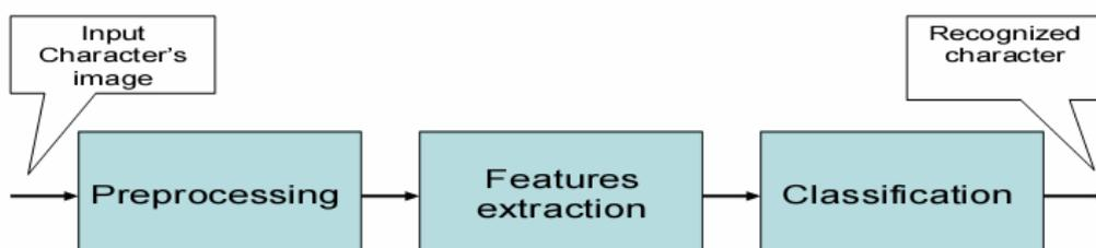
***(Figure-1) The typical OCR block diagram***
